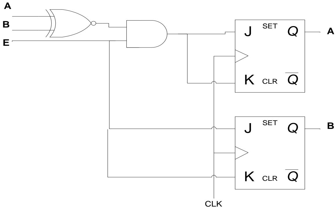
This sequential circuit behaves like a 2-bit up-down-counter, with E the enable of the whole counter, and resets when it finishes counting , when X=1, it behaves like an up-counter, when X=0 ,it behaves like a down-counter.
